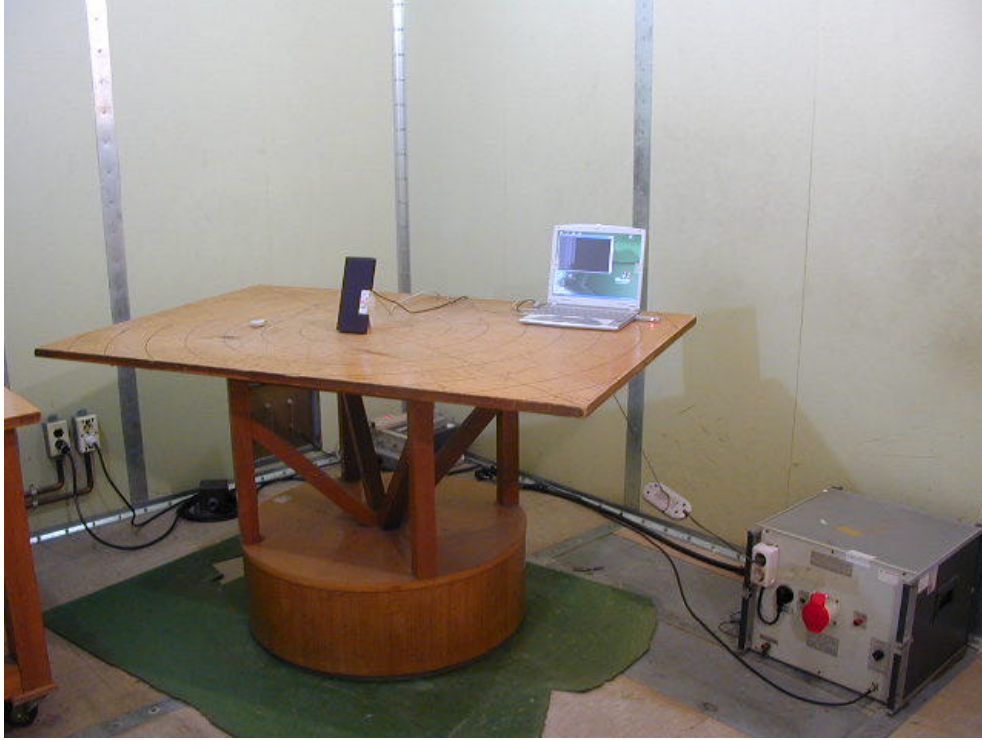
LINE CONDUCTED SETUP PHOTOGRAPH - FRONT VIEW
