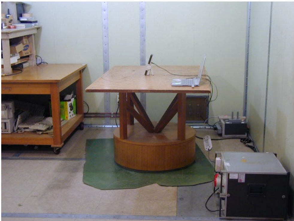
LINE CONDUCTED SETUP PHOTOGRAPH - REAR VIEW
