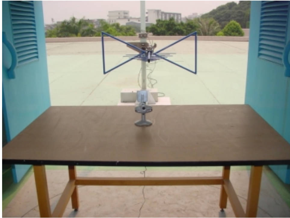
Photo7 Test Setup for Radiated Disturbance Test(Transmitter Front View)
