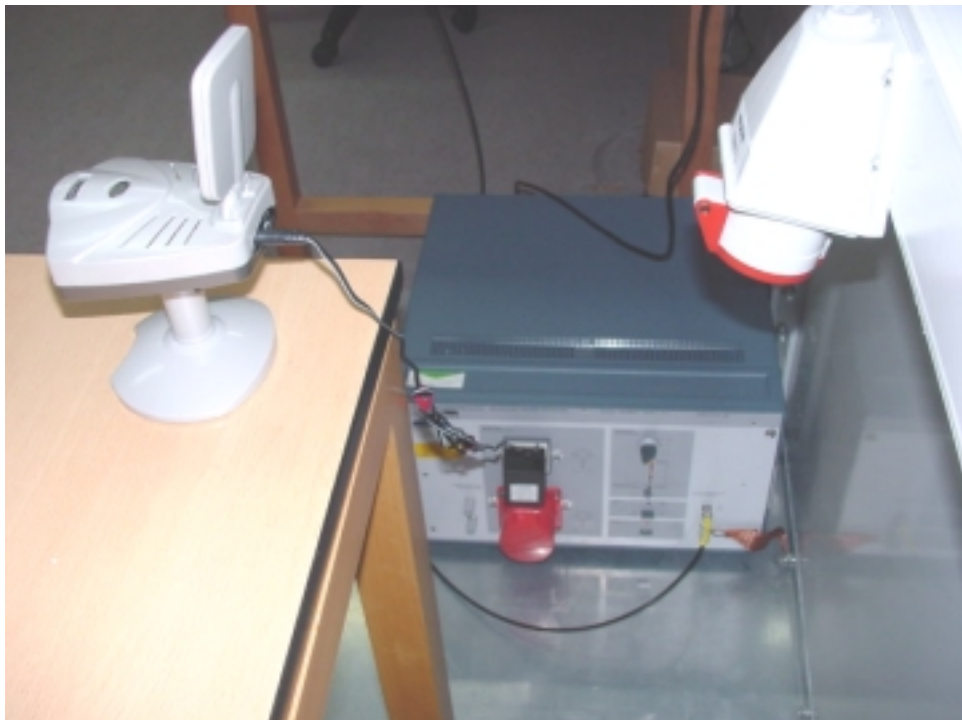
Photo4 Test Setup for Conducted Disturbance Test(Transmitter Rear View)
