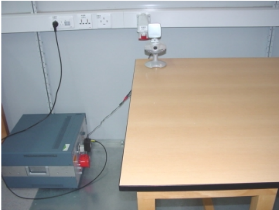
Photo4 Test Setup for Conducted Disturbance Test(Transmitter Rear View)
