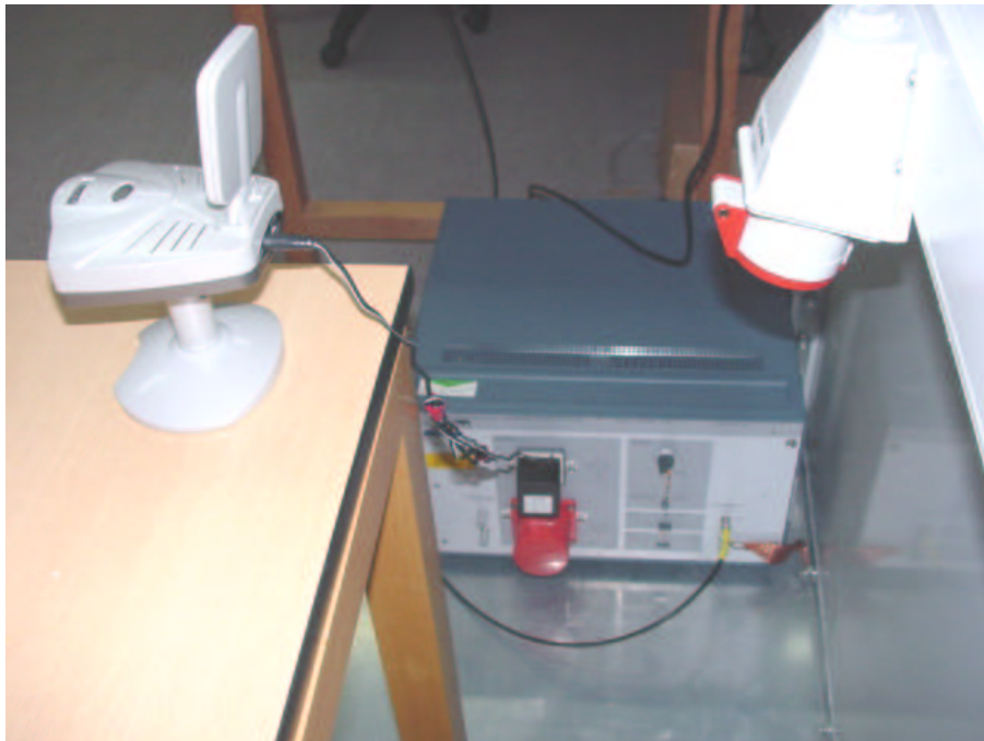
Photo2 Test Setup for Conducted Disturbance Test(Transmitter Rear View)
