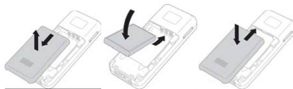
Figure 4. Installing the battery on a T1000 phone
