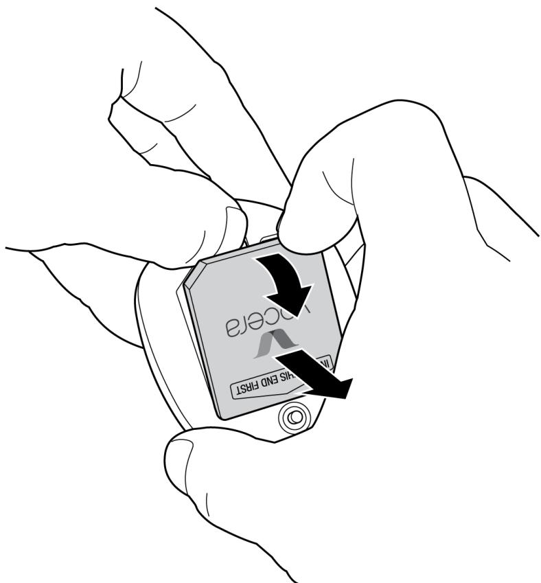
2. Insert the battery into the charger, and press the battery down.
