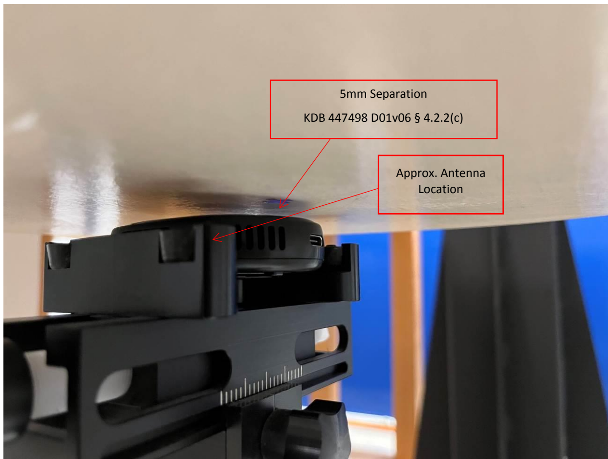
SAR Testing On Front Side
