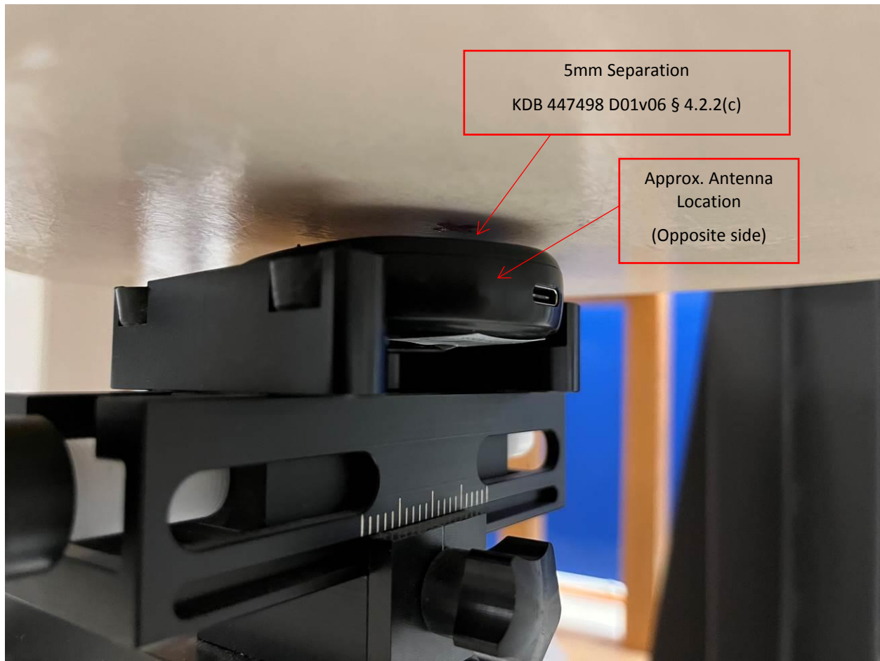
SAR Testing on Back Side
