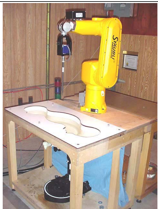
DASY4 System with SAM Phantom and device holder
