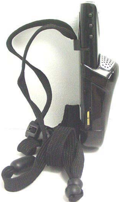
Left Side of Badge with Speaker Horn and Lanyard
