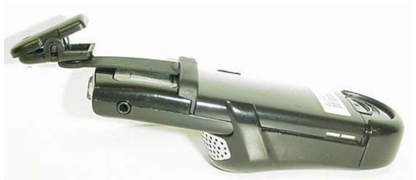
Back Side of Badge with Speaker Horn and Universal Clip
