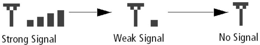
If the alert tone starts and stops as you move slightly, it means that you are at a location where the wireless network coverage begins.
