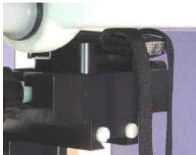
SAR Test Setup with Lanyard Accessory
