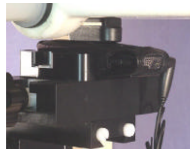
SAR Test Setup with Belt-Clip, Holster, & Headset Accessories
