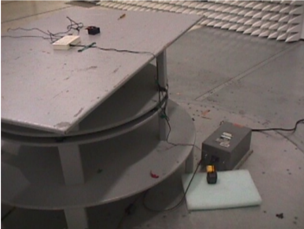
Conducted Emissions Test Configuration
