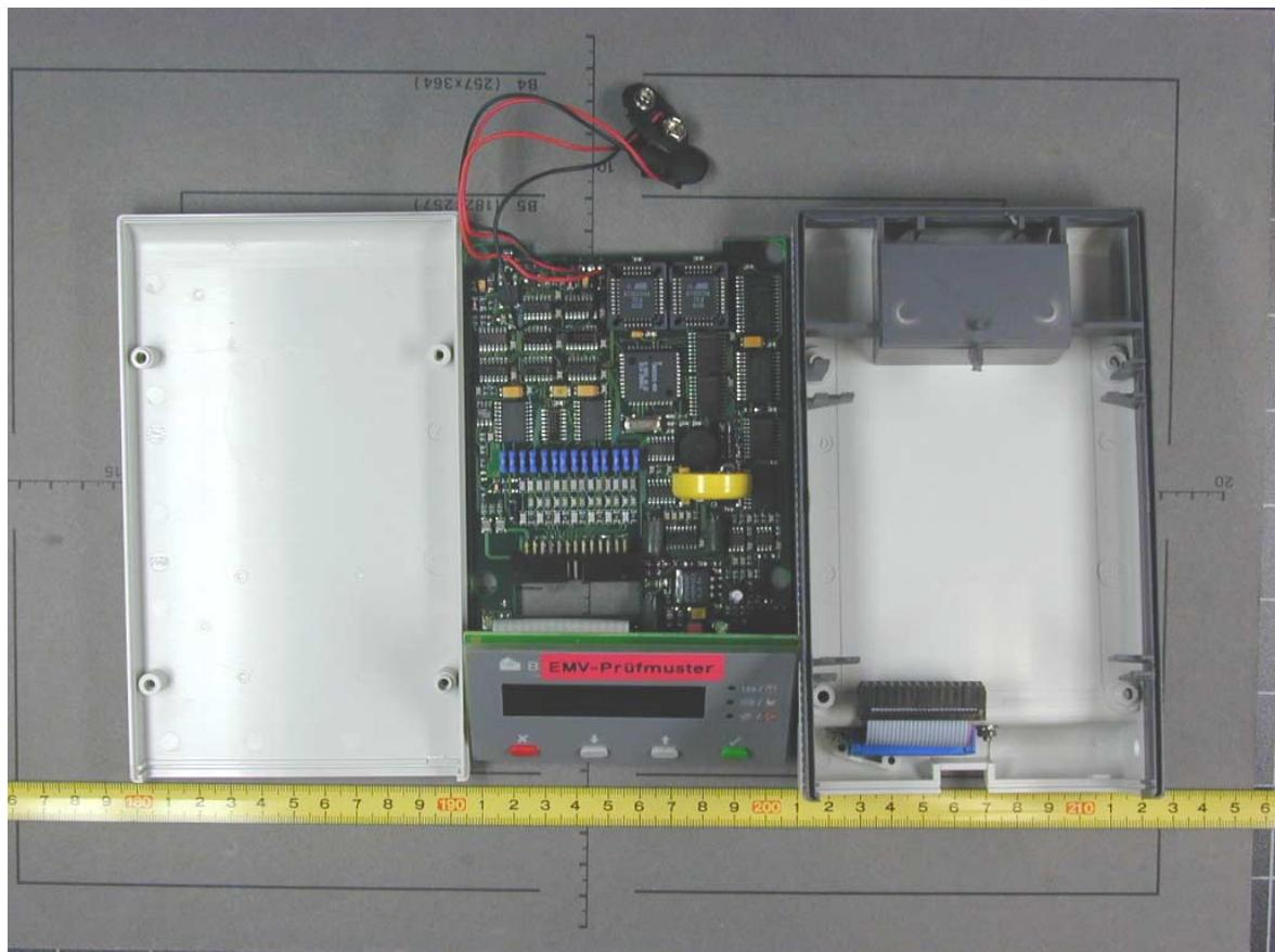
**Photo No. 6****Top view of printed board with internal antenna**
