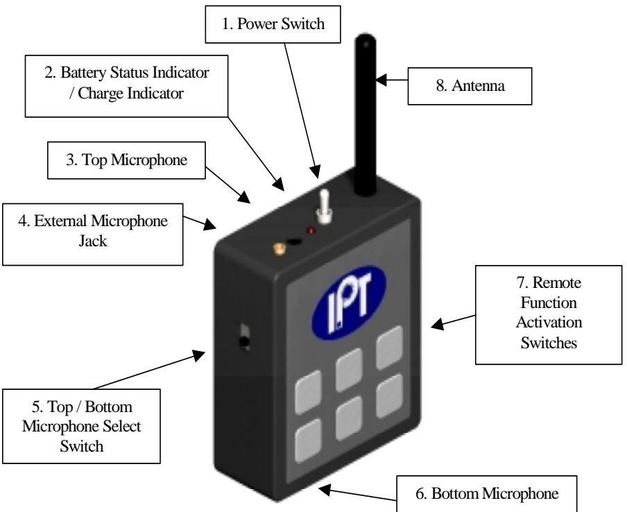
1. Power Switch – To check battery status, momentarily push switch lever towards the antenna. The LED next to the switch will glow RED when the battery is charged adequately to operate transmitter. To turn transmitter ON, push switch lever towards the LED and microphone connector.
