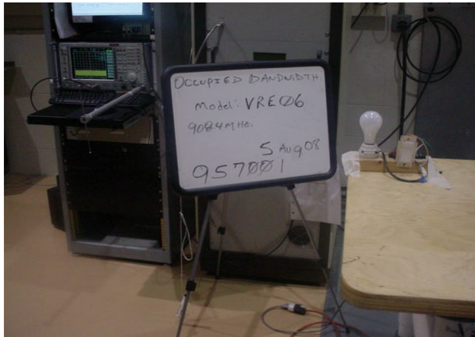
Figure 6 Test Setup for Occupied Bandwidth
