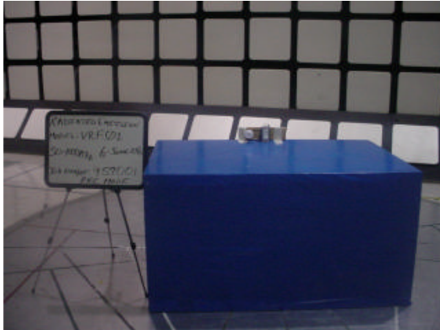
Figure 25 Test setup for Radiated Emissions 30 to 1000MHz– VRF01
