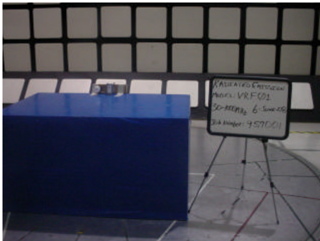
Figure 15 Test Setup for Radiated Emissions 30MHz to 1000MHz– VRF01
