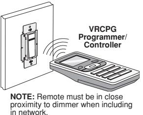
**NOTE:** Remote must be in close proximity to dimmer when including in network.
