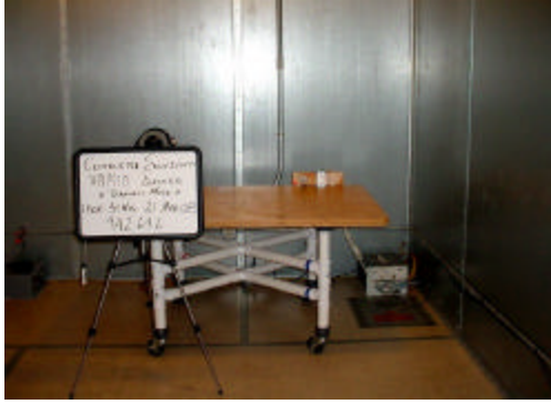
Conducted Emissions Set Up 150KHz to 30MHz
