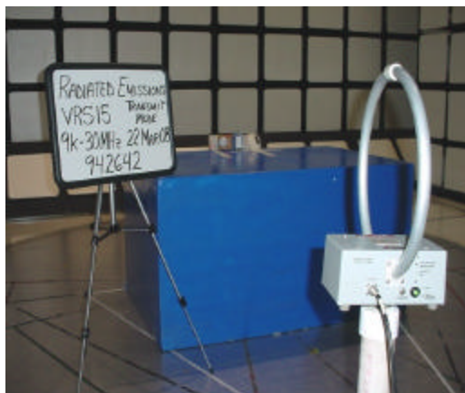
Radiated Emissions Set Up 9KHz to 30MHz
