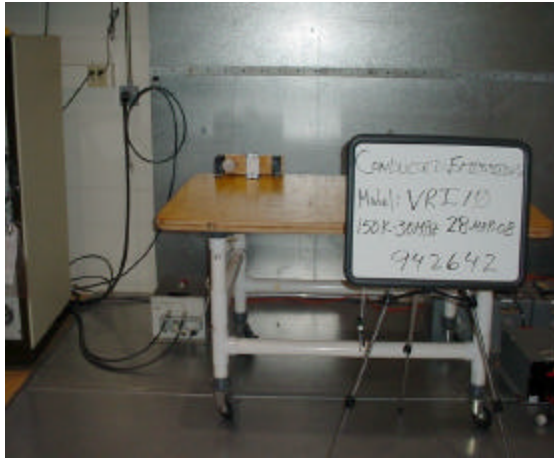
Conducted Emissions Set Up 150KHz to 30MHz
