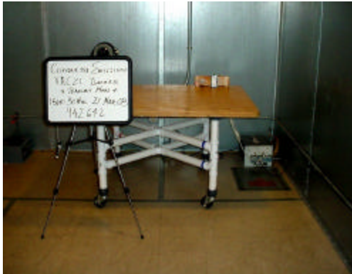
Conducted Emissions Set Up 150KHz to 30MHz
