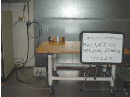
Conducted Emissions Set Up 150KHz to 30MHz
