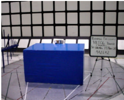
Radiated Emissions Set Up 30MHz to 1000MHz
