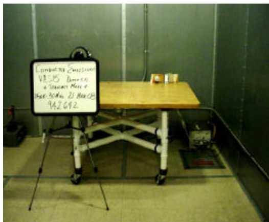
Conducted Emissions Set Up 150KHz to 30MHz
