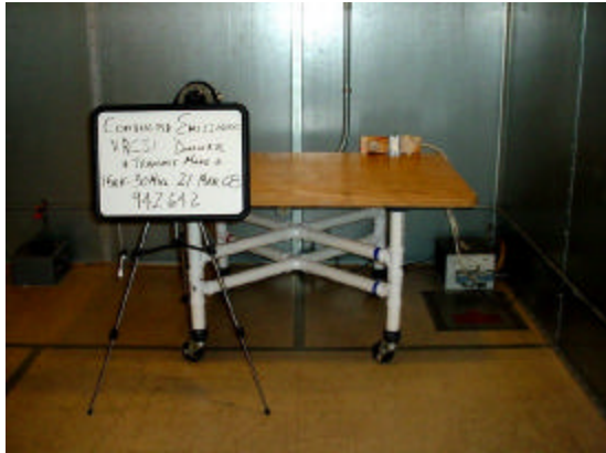
Conducted Emissions Set Up 150KHz to 30MHz
