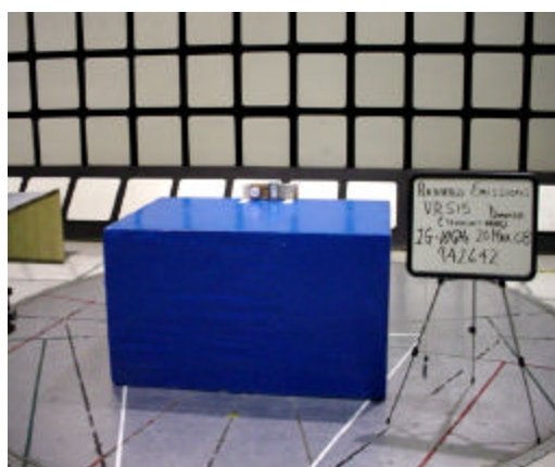
Radiated Emissions Set Up 1GHz to 10GHz
