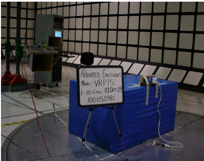
Figure 35: Test setup for Radiated Emissions
