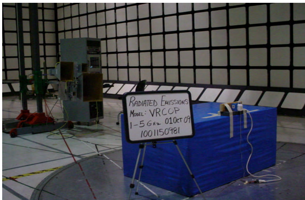
Figure 45: Test setup for Radiated Emissions
