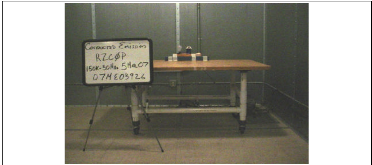
Figure 1 Test Setup for Conducted Emissions
