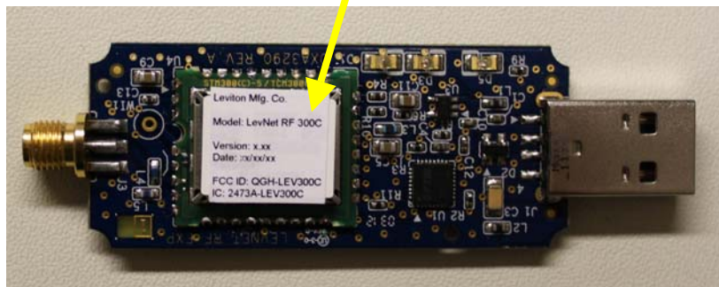
Figure 8. U4 (TCM300C) with modular label attached
