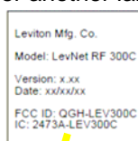
Figure 7. Module Label affixes to U4, TCM300C IC
