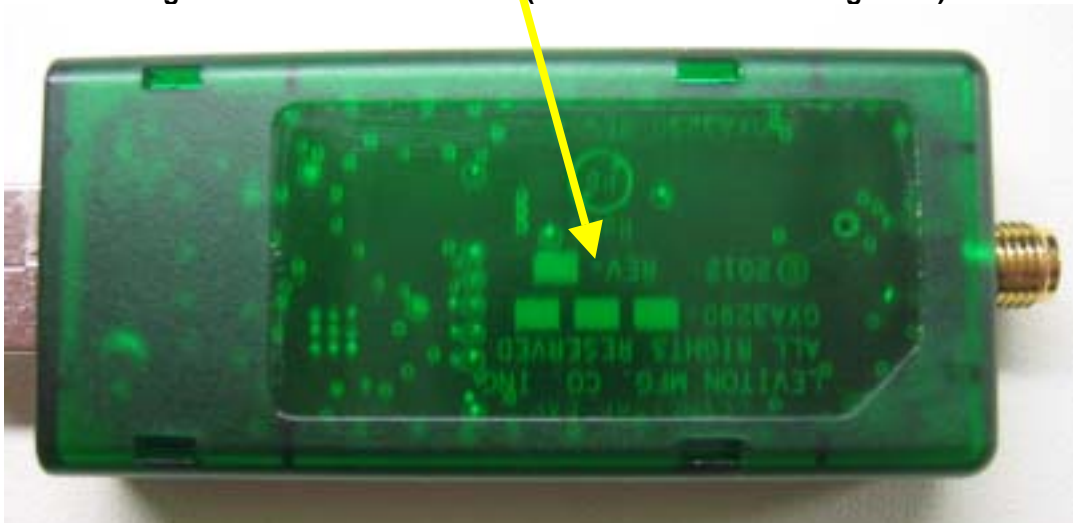
Figure 4. Back of WSCOM-03W: Label affixes to non-textured surface
