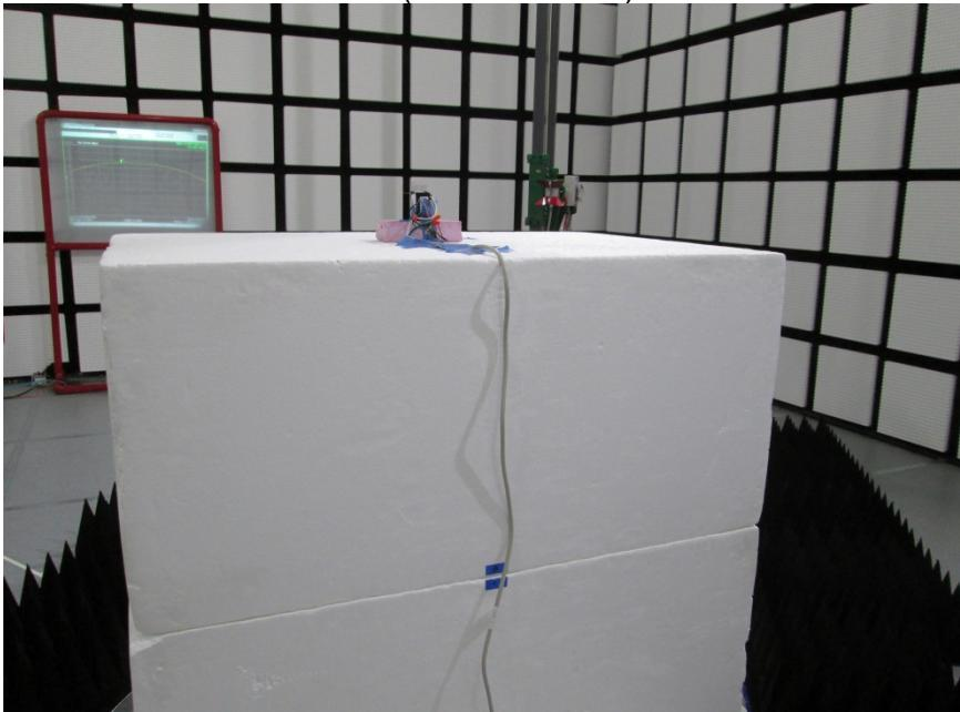
**RADIATED RF MEASUREMENT SETUP (ABOVE 18 GHz)**
