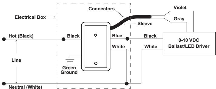
**b. LU20S Wiring Diagram**
