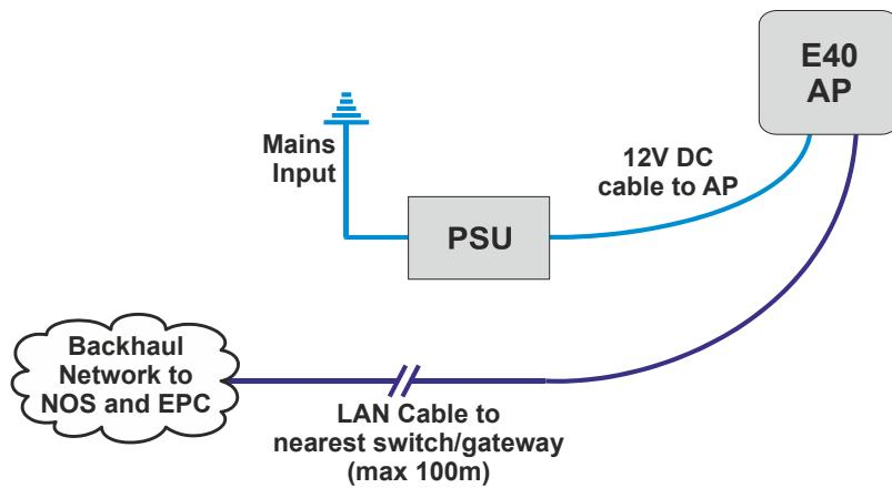
A mains socket providing power to the AP must be within reach of the cabling included with the PSU. This is typically less than 1.5m. The PSU for the E40 AP is supplied.
