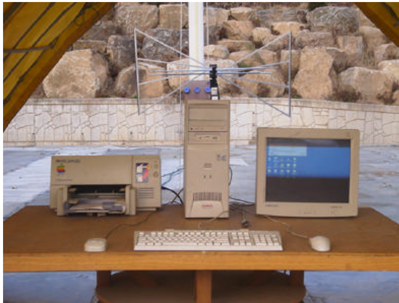
Photograph 1 : Setup for radiated Emissions
