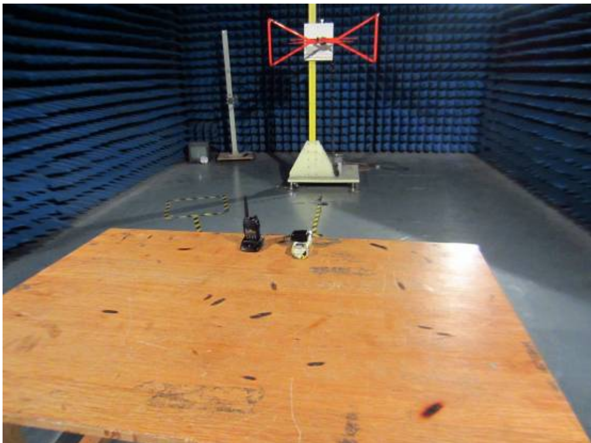
Radiated Emission Setup Photo
