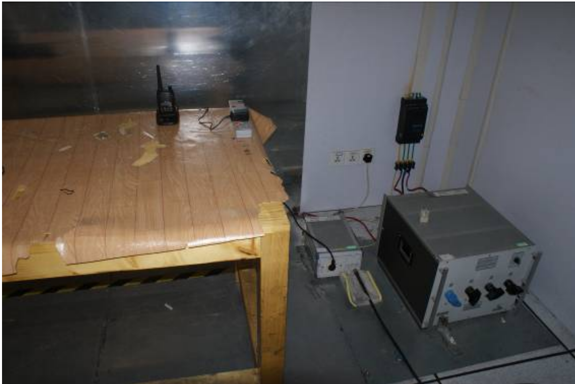
Conducted Emission Setup Photo
