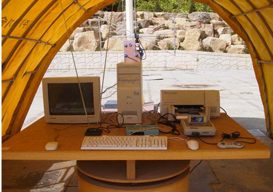
Photograph 1 : Setup for radiated Emissions
