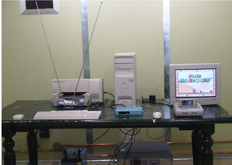
Photograph 2 : Setup for Conducted Emissions
