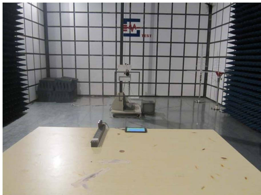
**Spurious Radiation Test Setup (30MHz to 1G)**
