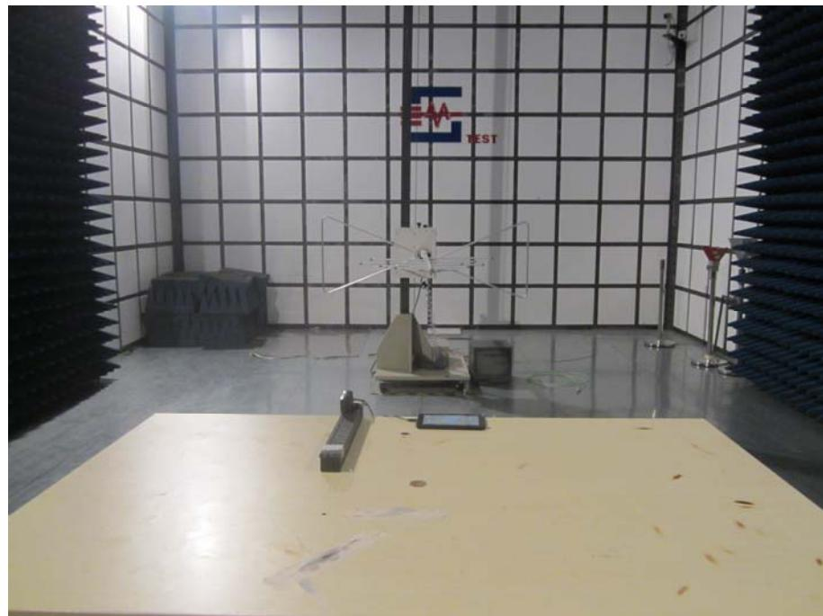
**Spurious Radiation Test Setup (Above1G)**
