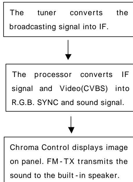
\* Power and MICOM supply power to the circuit and control parts.
