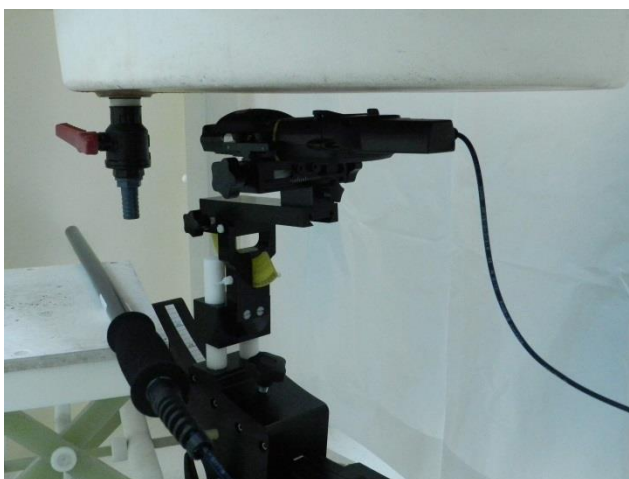
Back with With external RFID antenna, Test Separation 1.5 cm
