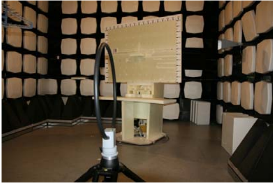
Picture 2. FCC Part 15C Radiated emissions, FM TX
