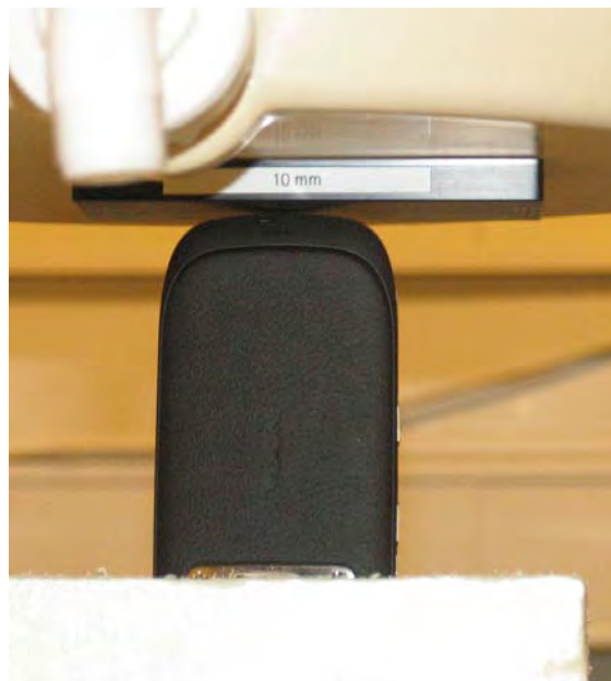
Photo of the device positioned for WR mode measurement – bottom edge facing phantom. The spacer was removed before the start of the measurements.
