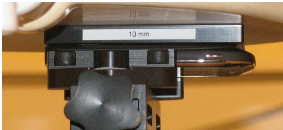
Photo of the device positioned for WR mode measurement – back facing phantom. The spacer was removed before the start of the measurements.
