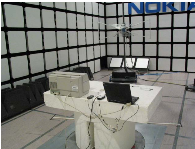
Picture 3. FCC Part 15B Radiated emissions
