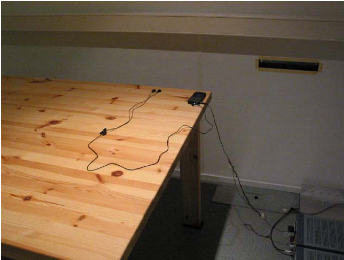
Picture 4. FCC Part 15C AC powerline conducted emissions
