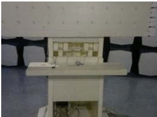
Picture 3. FCC Part 15B Radiated emissions
