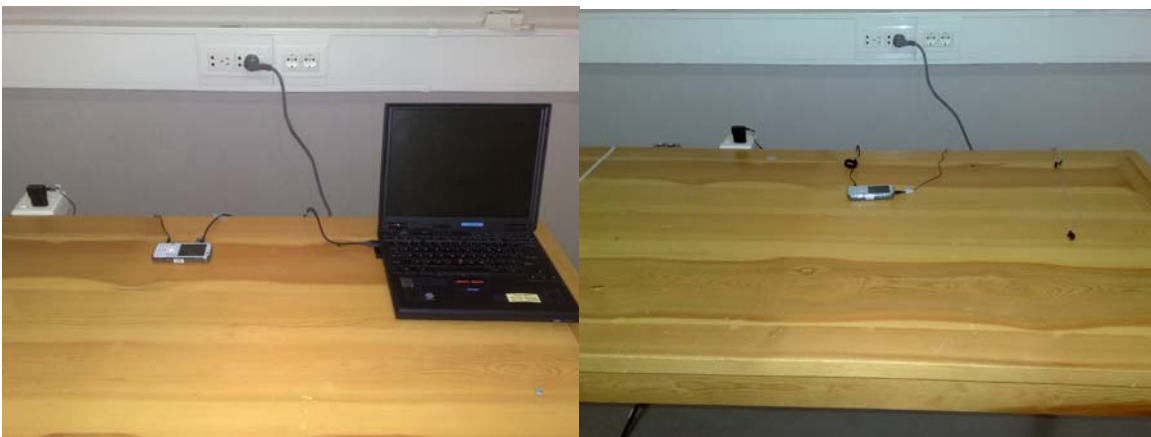
Picture 4 AC powerline conducted emission measurement GSM RX/ Bluetooth TX
