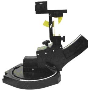
Device holder supplied by SPEAG
