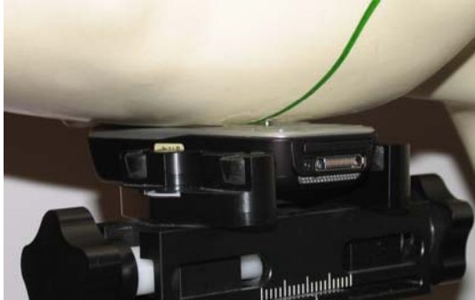
Photo of the device in "cheek" position
