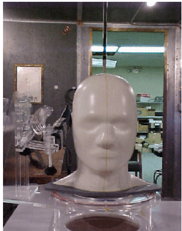
Figure S14. Configuration #14 - Tilt ( 15^{\circ} ) position, left side, GPS Out, 900 mAH Battery
