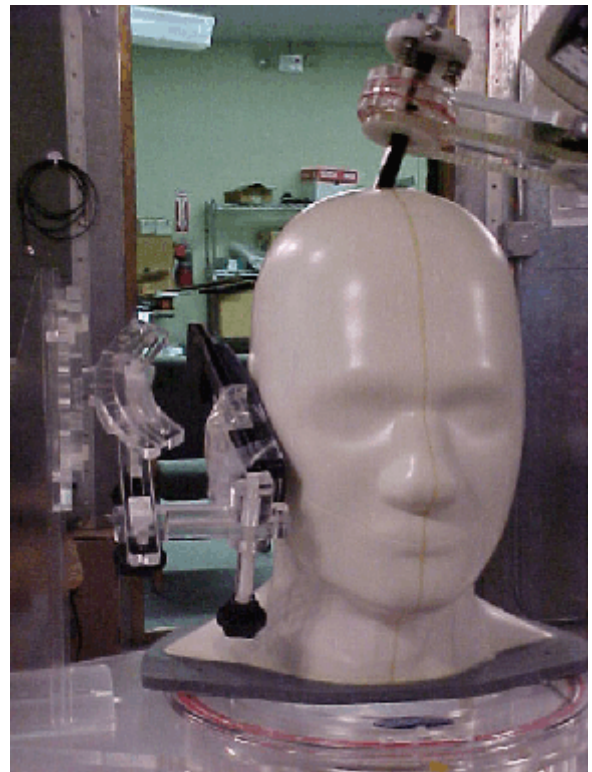
Figure S16. Configuration #16 - Cheek ( 0^\circ ) position, left side, GPS Out, 900 mAH Battery
