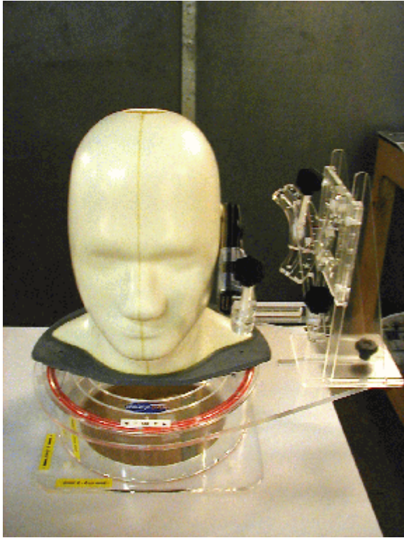
FigureS7. Configuration #7 - Cheek ( 0^{\circ} ) position, right side, GPS In, 900 mAH Battery
