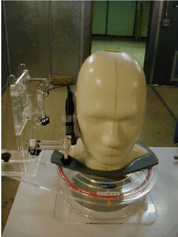
Figure S11. Configuration #11 - Cheek (0°) position, left side, GPS In, 1200 mAH Battery
