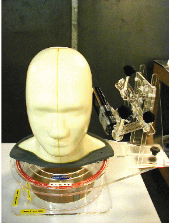
Figure S5. Configuration #5 - Tilt ( 15^{\circ} ) position, right side, GPS In, 900 mAH Battery
