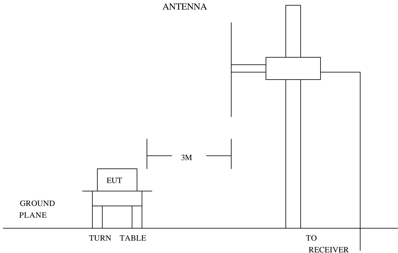
**4 . 3 RADIATED TEST SET-UP**
