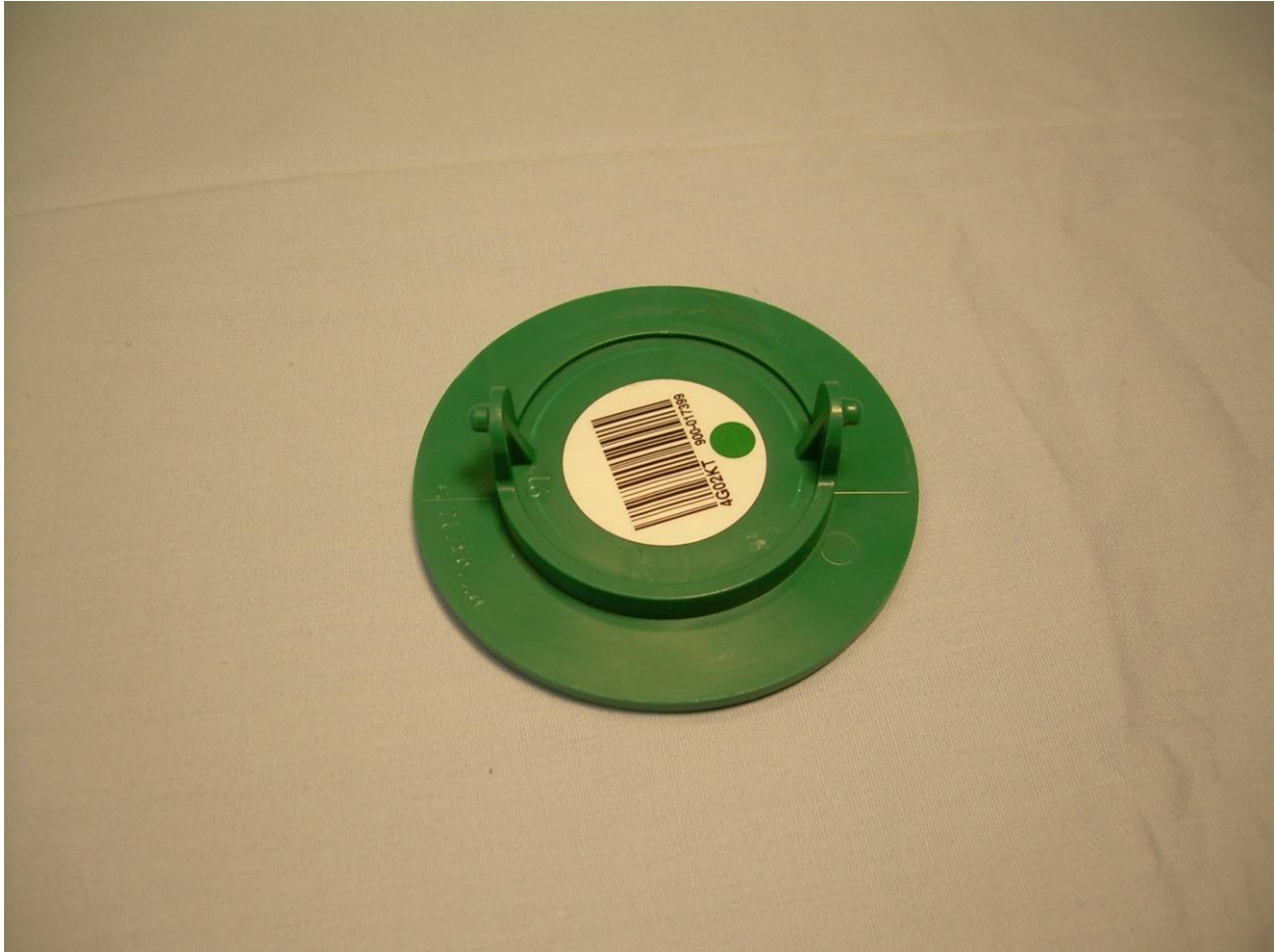
Photograph 16 – Bottom View of the RFID Tag
