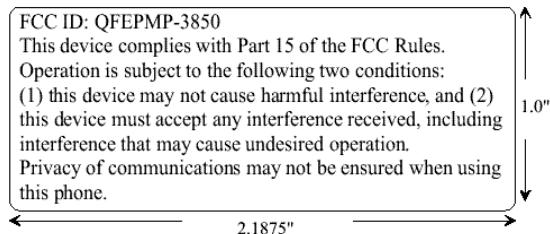
Specifications: Text is black or white in color and is left justified. Labels are silk-screened and shall be "permanently affixed" at a conspicuous location on the EUT.
