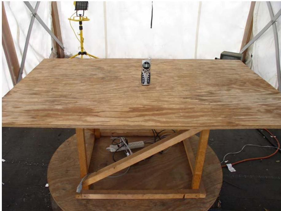
**Handset Radiated Emission - Rear View**
