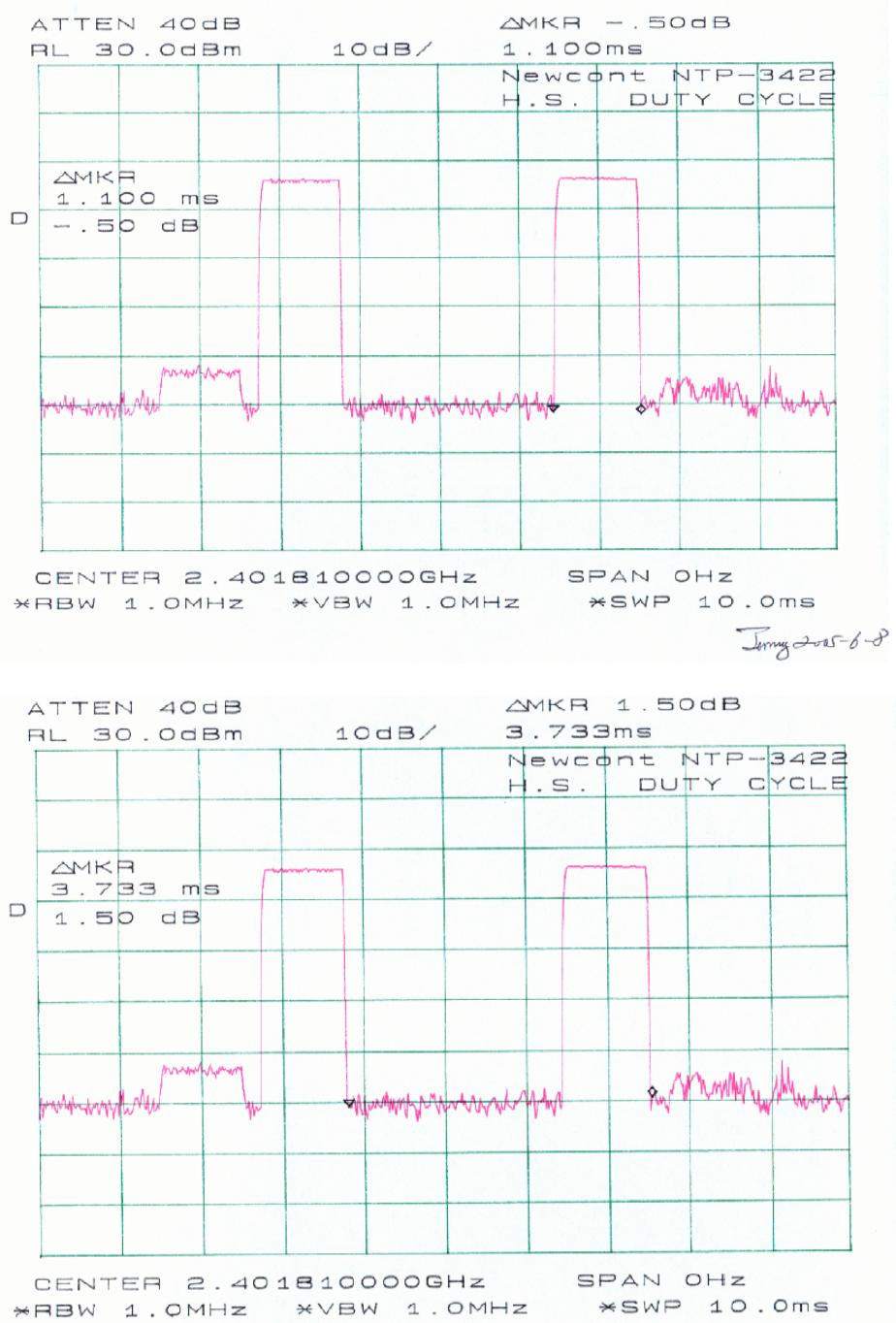
$$\text{Duty Cycle} = \text{TX}_{\text{on}} / (\text{TX}_{\text{on}} + \text{TX}_{\text{off}}) = 1/13.733$$
