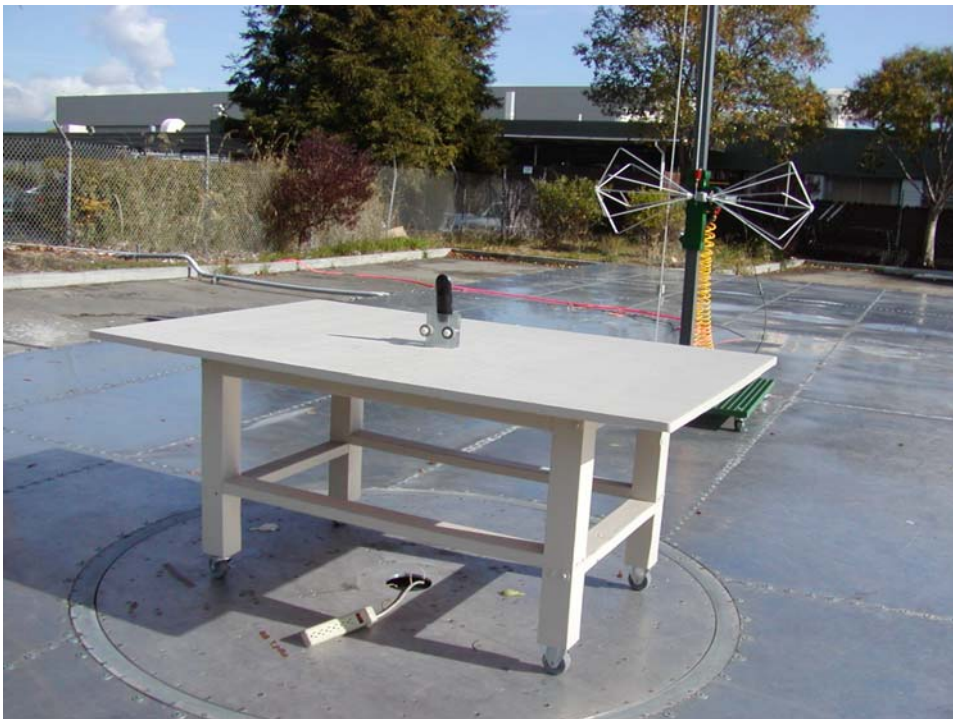
Handset Radiated Emission - Rear View
