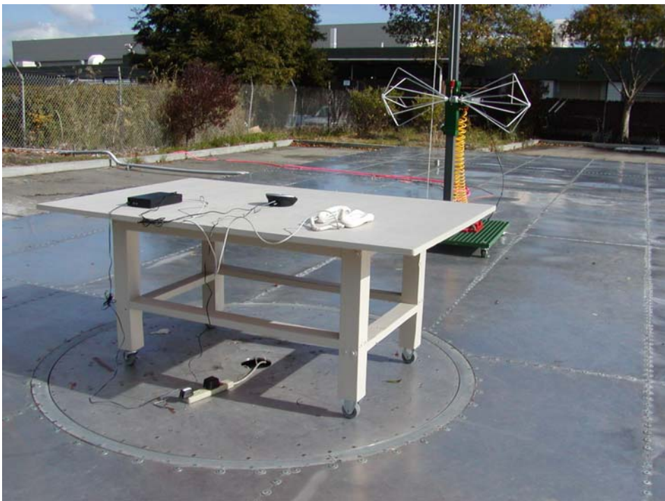
Base Radiated Emission – Rear View
