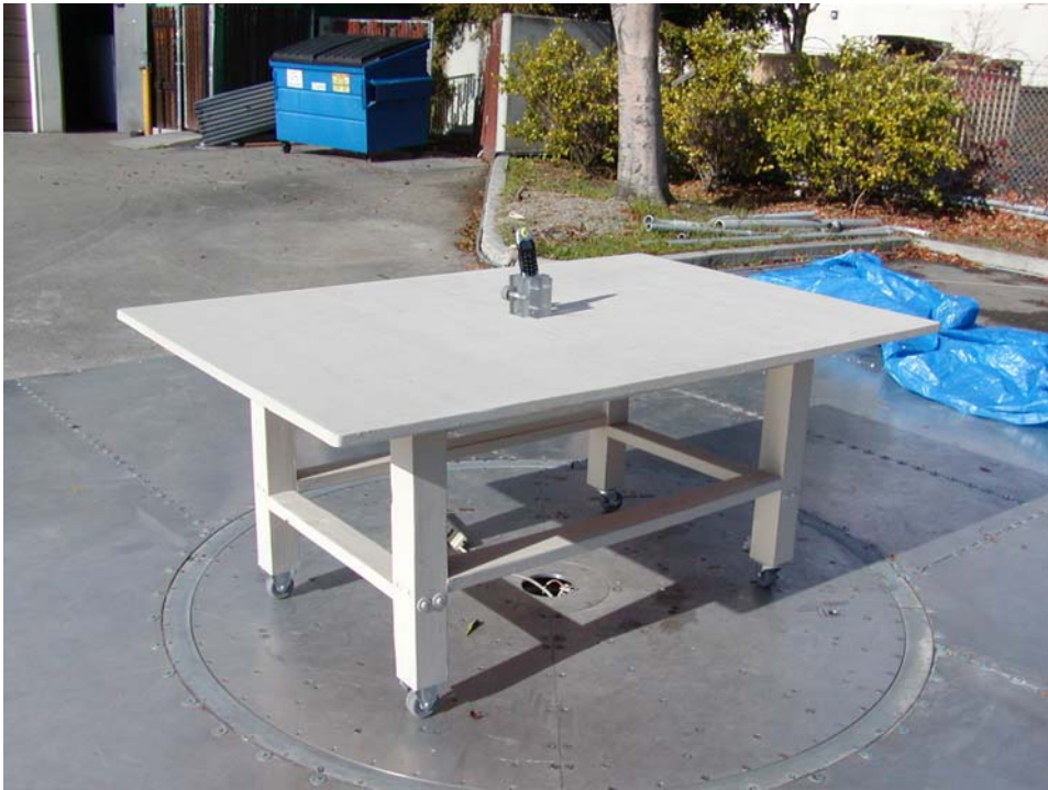
Handset Radiated Emission - Front View
