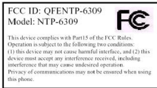
**Specifications:** Text is black or white in color and is left justified. Labels are silk-screened and shall be “permanently affixed” at a conspicuous location on the EUT.
