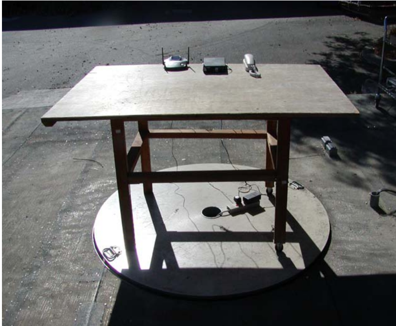
EUT – Base Unit Radiated Emission Set Up – Front View
