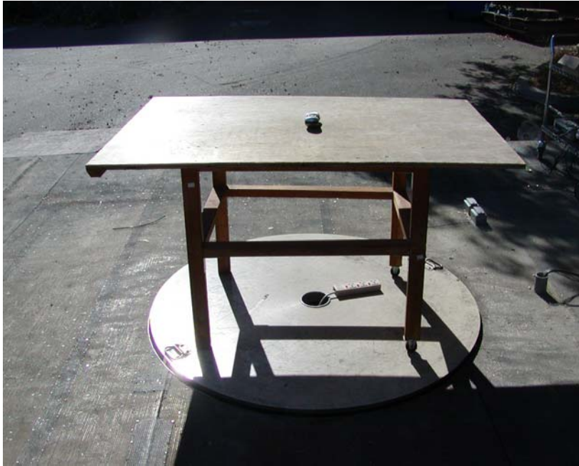
EUT – Handset Unit Radiated Emission Set Up – Front View
