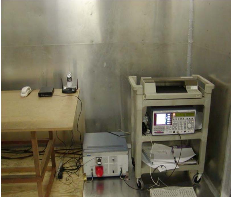
EUT – Conducted Emission Set Up - Front View
