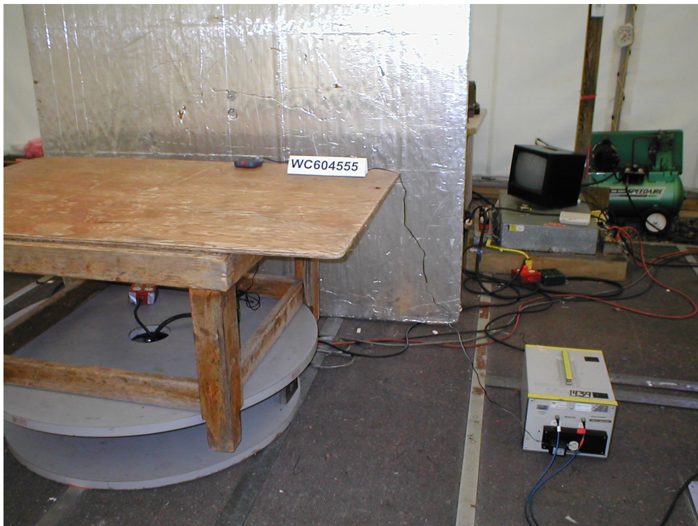
Test-setup photo: Conducted Emissions Model CLP-BMT1
