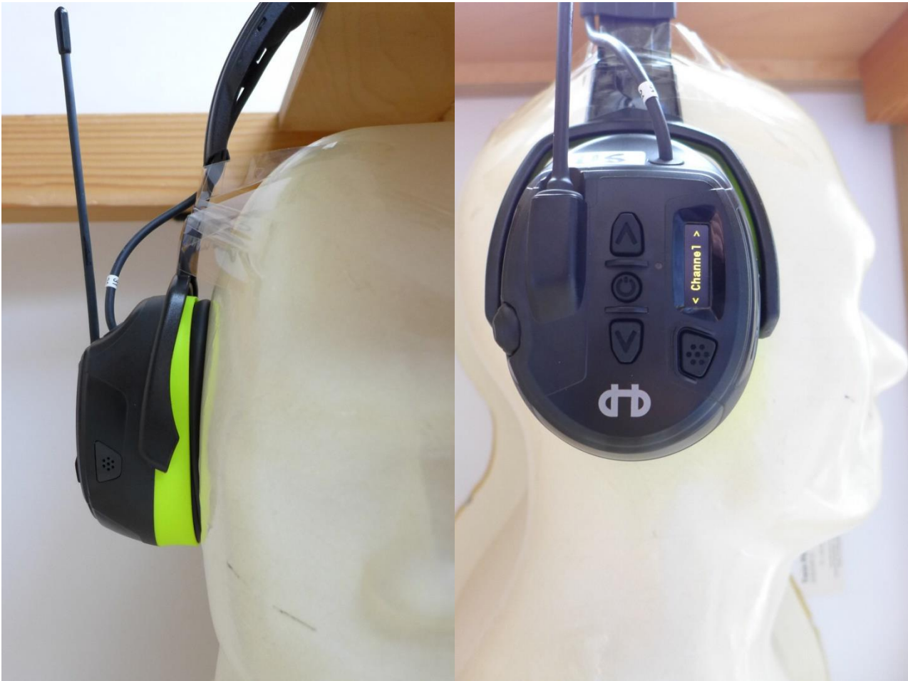
Pic. 5: Test position right side of DUT, cheek right.
