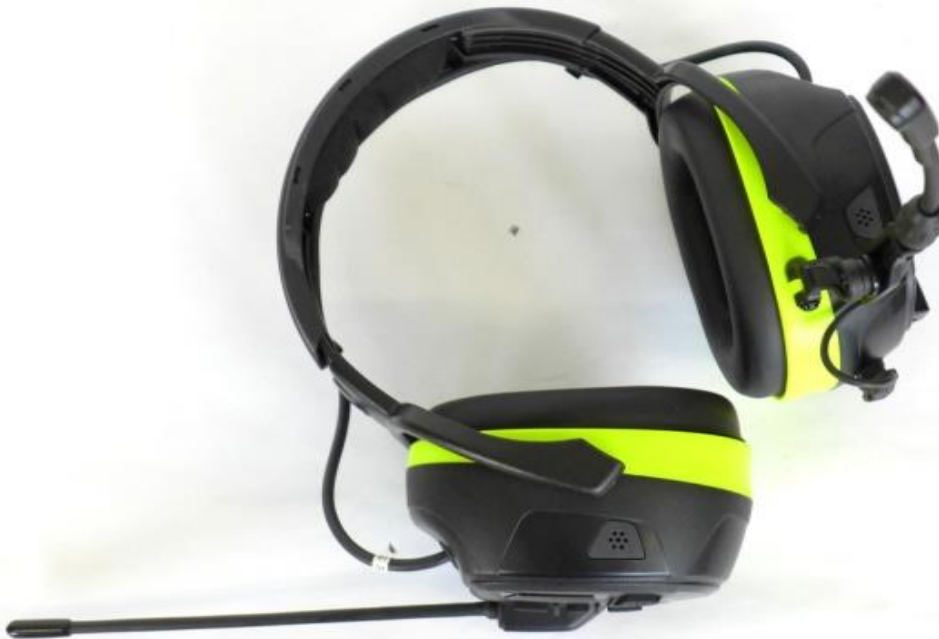
Fig. 3: Antenna location on the right earpiece of the DUT.
